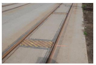
The APT-WORM system (Wheel Out of Roundness Measurement) is specifically developed for the detection of flats and out of roundness of wheels on heavy and light rail vehicles.
